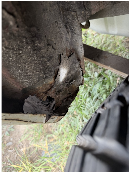
IMG_0592.jpeg — Lower wheelhouse or adjoining rear sheetmetal with rust-through.
