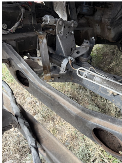
IMG_0597.jpeg — Front rack/crossmember and modified mounting arrangement.
