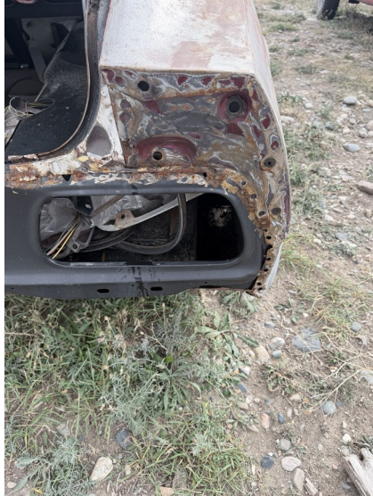
IMG_0579.jpeg — Rear lamp opening and trunk-corner corrosion/previous work.
