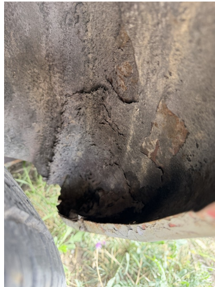
IMG_0593.jpeg — Lower rear sheetmetal with a large irregular perforation.
