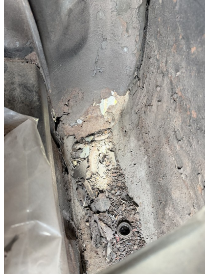
IMG_0590.jpeg — Interior rear cavity with extensive perforation and scale.
