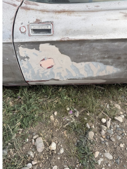
IMG_0581.jpeg — Lower door showing exposed filler and repair layers.
