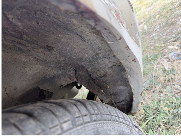
IMG_0587.jpeg — Wheelhouse opening with deteriorated metal and coating.
